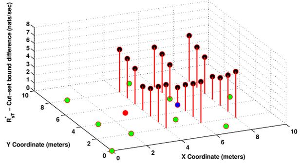
Fig. 3.  $|T| = 9$  case with green receivers, red source and blue as the optimal relay position. The optimal  $R_{sT}$  and cut set bound difference (in nats/sec) is calculated for 21 positions and is the lowest at the optimal relay position (blue). We assume  $\frac{P_s}{N_0} = \frac{P_r}{N_0} = 1$  (normalized) and  $\alpha = 4$ .
